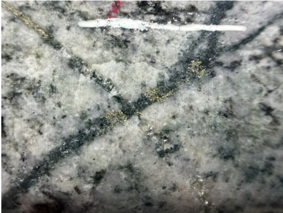
Figure 4. TCDH-006, 369 meters. Crosscutting high-temperature quartz veinlets carrying chalcopyrite, hosted in potassic-altered intramineral porphyry. Selected interval. Chalcopyrite identified visually by hand lens. Photograph: Quimbaya Gold Inc.
